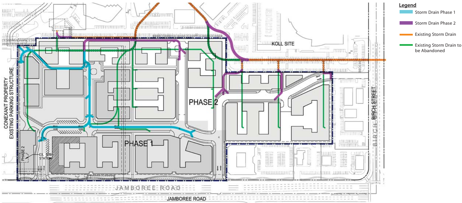
Figure 6-4: Storm Drain Concept Note: All plans are for illustrative purposes only
