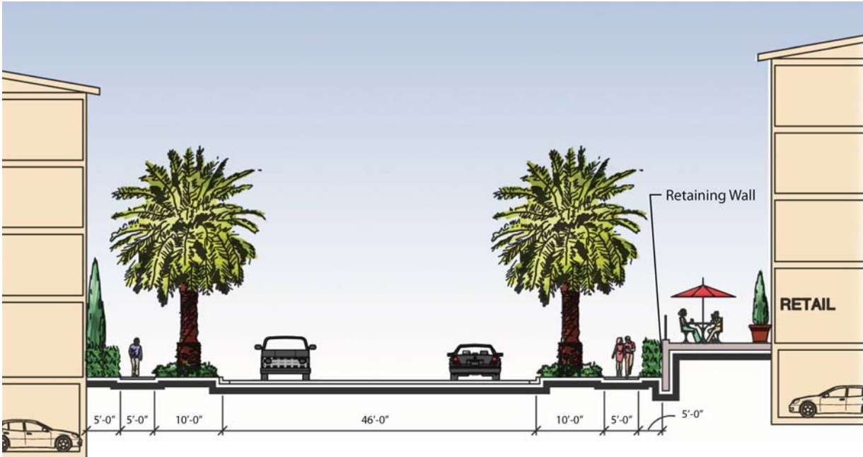
Figure 6-7: Section A - Entry Drive Note: All plans are for illustrative purposes only
